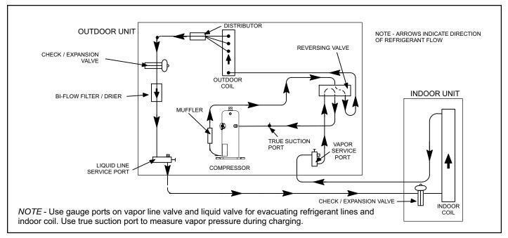
Figure 21. Heat Pump Cooling Cycle
